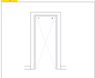
Check that the door opening is square by measuring the door frame diagonally. If the frame is out of square, you may have to order a slightly larger door and trim it to size. A trimming allowance of up to 5mm is allowed on most doors.
