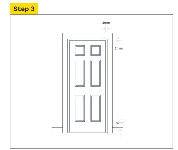
Keep in mind that approximately 3mm clearance is required for the top and sides of the door and 5mm for the bottom, above the floor covering or door frame sill.
